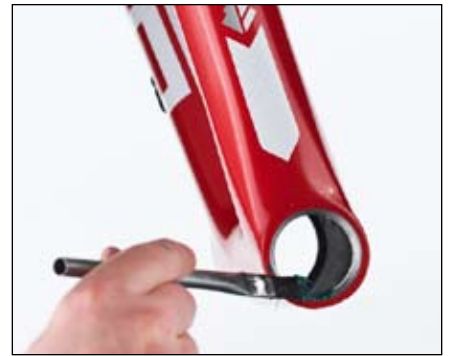
Figure 7. Greasing upper bearing saddle
